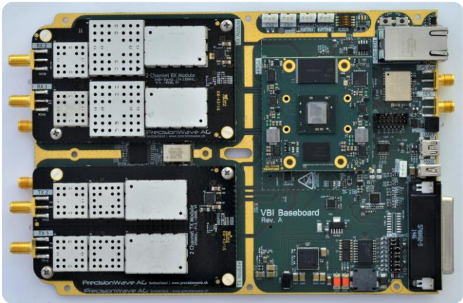
Modular, broadband RF Interfaces (up to 150MHz RX- and 600MHz TX-bandwidth) make our system ready for you customized frequency needs. Contact us with your specifications.
