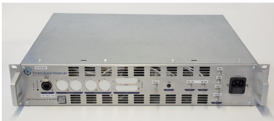
19" rack version as all-in-one solution: X-band radar, PSU, fuse and thermal management
